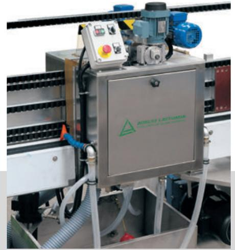
The washing machine applied to the edging machines and beveling machines outlet conveyor allows the complete cleaning and drying of the processed edges of the glass sheets.
